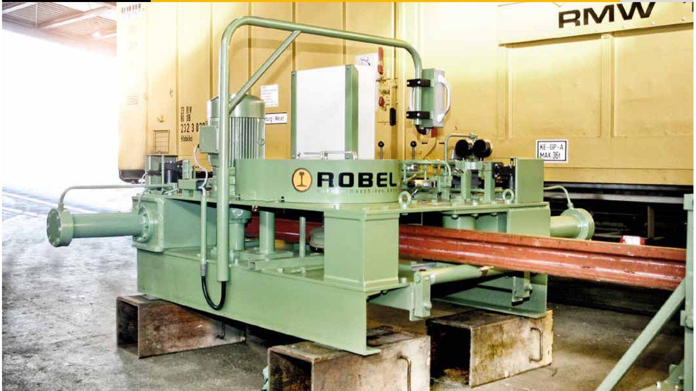
4 Roller-type Rail Bending Machine with hydraulic (roll) feed for bending grooved rails and vignol rails.
